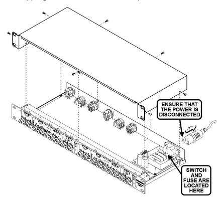
Accessing the internal power switch and fuse
