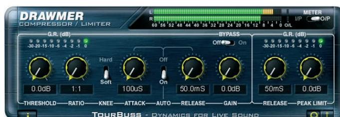
The Tourbuss Compressor combines aspects of both the traditional ratio style compressor and the soft knee approach, making it equally adept at creative work and unobtrusive level control. Many advanced facilities that enable quick setup, predictable results and a musical analogue style response have been incorporated, including:
