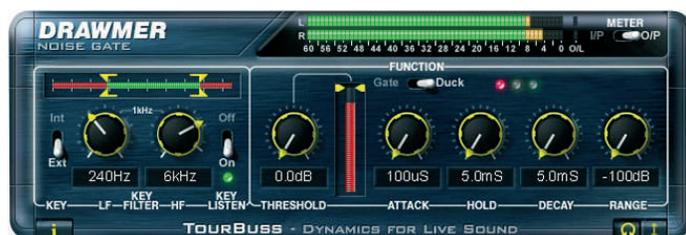
The Tourbuss Noise Gate is based on the industry standard Drawmer DS201, the world's first 'frequency conscious' Noise Gate. The DS201 redefined the role of gating in both the recording studio and live sound environments and transformed what was previously a simple on/off device into a powerful production tool. This unique design approach resulted in a gate that opens to user defined frequency bands, as well as signal level and in addition provides sophisticated envelope shaping.
