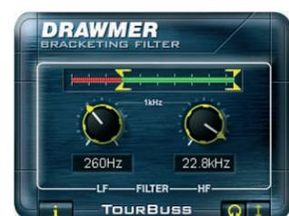
The Tourbuss Bracketing Filter provides Low and High 12dB per octave filters that attenuate any unwanted frequencies. A Bracketing Filter is most widely used to remove signals created at high or low frequencies that bleed into the source.
