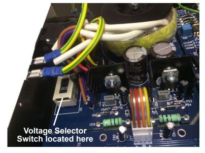
fig.2 The Voltage Selector Switch
